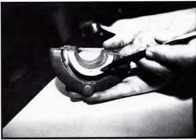
Here's one of the thrust surfaces on a rear main bearing cap. The other is on the opposite end of the cap.
